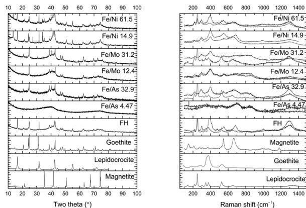
**Fig. 1** Powder X-ray diffraction spectra (left) and micro-Raman spectra (right) of solid products reacted at a target pH of 8 for 7 days with 10 mM  $\text{Fe(II)}_{(\text{aq})}$ . Spectra of relevant standard materials are shown for comparison. For each reacted sample, two Raman spectra are presented to show the mixtures of phases found in the reacted sample.
